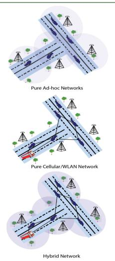
Fig 1. Three Architectures of VANET Pure Ad-hoc Networks, Pure Cellular /WLAN Networks, Hybrid Architecture
